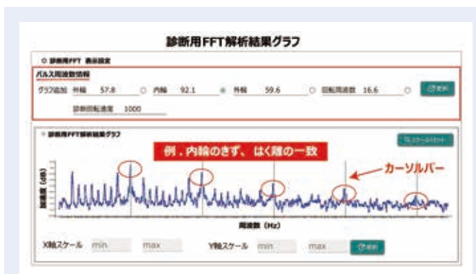
図3 ACOUSNAVI for Bearings (軸受診断アプリ)の解析結果グラフ Fig. 3 Analysis results graph from ACOUS NAVI for Bearings (bearing diagnostics app)
