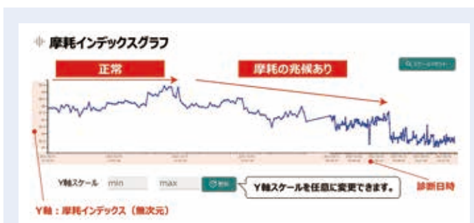
図4 ACOUS NAVI for Ball Screws (ボールねじ診断アプリ)の解析結果グラフ Fig. 4 Analysis results graph from ACOUS NAVI for Ball Screws (ball screw diagnostics app)
